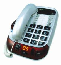
The Alto features an oversized backlit keypad, 10 one-touch memory buttons, and powerful speaker phone. It also has a loud adjustable ring and talking keypad.
